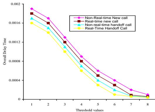
Figure 3: Average delay time versus threshold values
