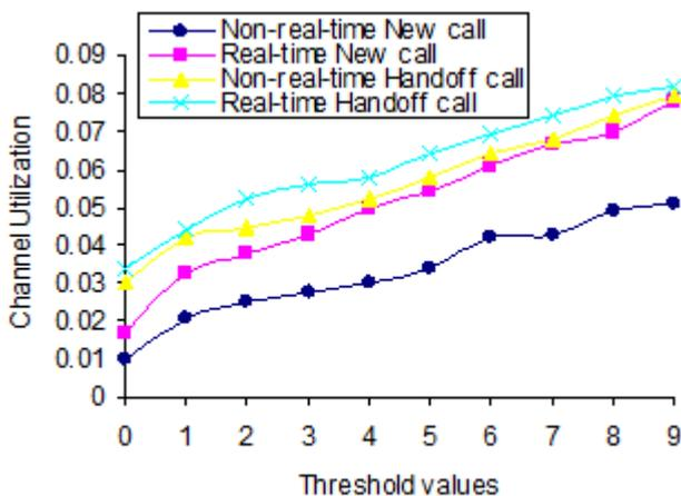
Figure 4: Channel utilization under different threshold values
