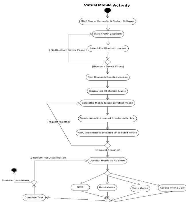
Figure 12: Activity diagram of virtual mobile
