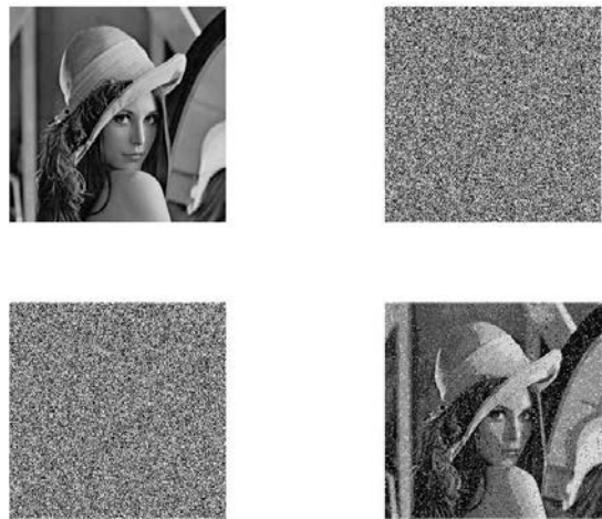
Fig. 4: Robust test for JPEG compression with quality=70, the upper left is the plain-image Lena, the upper right is the cipher-image, the lower left is the cipher-image attacked by JPEG compression, the lower right is the decrypted image for the attacked cipher-image.
