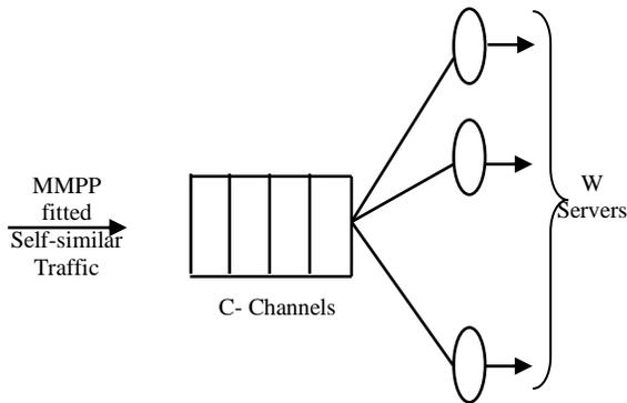
Figure 2. MMPP/M/W/C - The equivalent queuing model of WDM OPS depicted in Fig. 1
