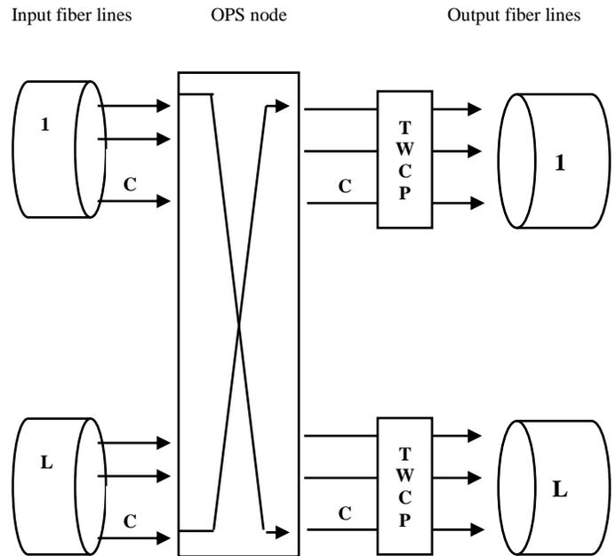
Figure 1. Architecture of SPL type of OPS node, 'L' I/O fiberlines, each with 'C' no. of channels and Tunable Wavelength Converter Pool (TWCP) of size 'W'
