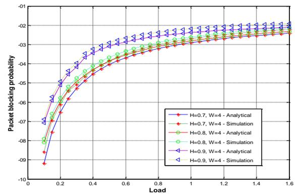
Figure 6. Comparison of packet blocking probabilities of MMPP/M/W/C when  $H=0.7$ ,  $0.8$  and  $0.9$ ,  $C=4$ ,  $W = 4$ ,  $W$  – number of wavelength converters.
