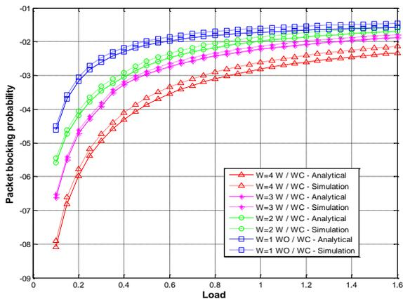
Figure 4. Packet blocking probabilities of MMPP/M/W/C, when  $H=0.8$ ,  $C=4$ ,  $W$  – number of wavelength converters,  $WO /WC$  – without wavelength conversion,  $W/WC$  – with wavelength conversion
