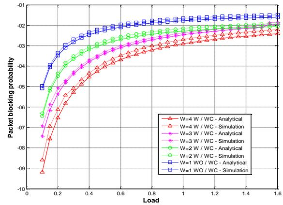
Figure 5. Packet blocking probabilities of MMPP/M/W/C, when  $H=0.7$ ,  $C=4$ ,  $W$  – number of wavelength converters,  $WO /WC$  – without wavelength conversion,  $W/WC$  – with wavelength conversion.
