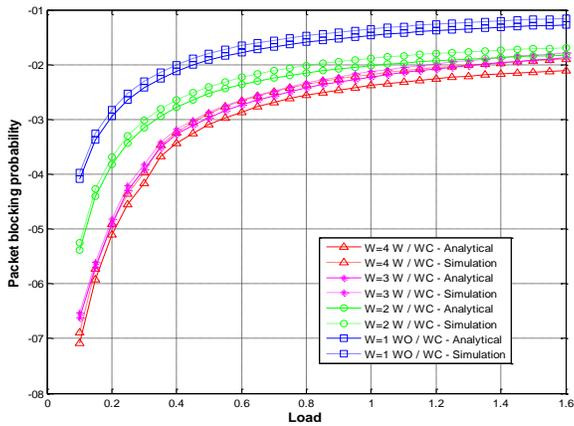
Figure 3. Packet blocking probabilities of MMPP/M/W/C, when  $H=0.9$ ,  $C=4$ ,  $W$  – number of wavelength converters,  $WO /WC$  – without wavelength conversion,  $W/WC$  – with wavelength conversion.
