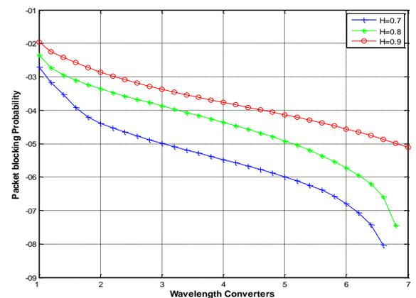
Figure 7. Comparison of packet blocking probabilities of MMPP/M/W/C against No. of tunable wavelength converters, when  $H=0.7$ ,  $0.8$  and  $0.9$  and the Load is  $0.85$ .
