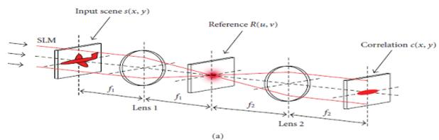
Figure 3: Optical setup
