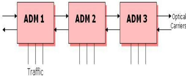
Figure 6: Configuration of SONET/SDH Networks
