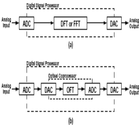
Figure 5: Processing Analog Signal with a Digital Signal Processor
