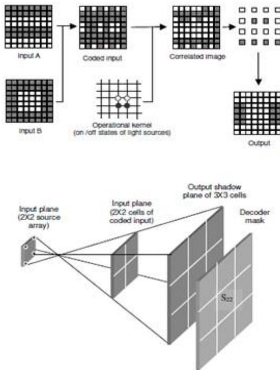
Figure 2: Optical logic processing architecture
