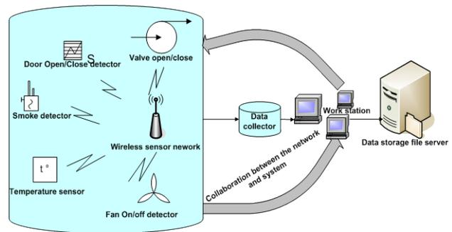
Figure 3. Collaboration between network and the system.
