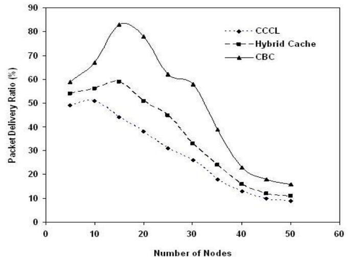
Fig. 2 Comparison of CCCL, Hybrid Cache and CBC in terms of Packet Delivery Ratio
