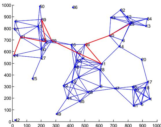
Figure 5: Network Topology Showing Shortest Route Under Two-Constrained Dijkstra Algorithm
