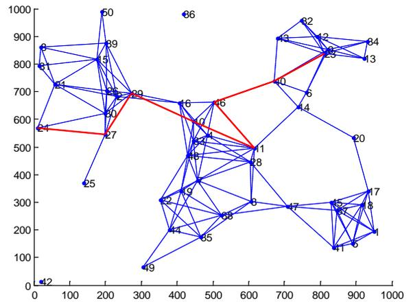
Figure 6: Network Topology Showing Shortest Route Under Three-Constrained Dijkstra Algorithm
