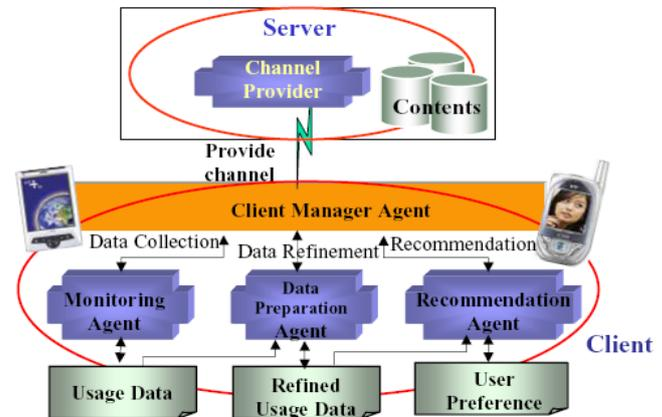
**Figure 6: Overall Architecture of System for Providing Personalized Channel Recommendation in Mobile Environment**
