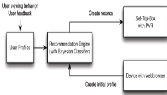
**Figure 2: Architecture of Personal Video Recorder (PVR) Implementation**
