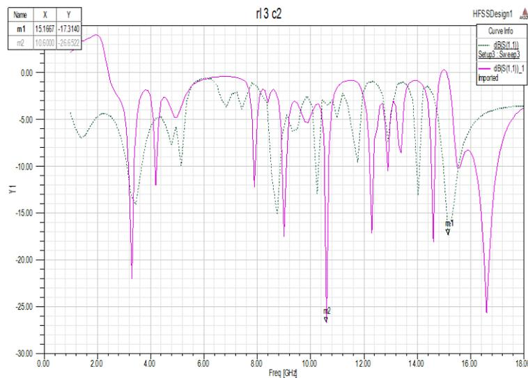
Figure 3: Return Loss Plot (1GHz – 18 GHz)
