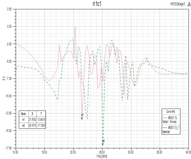
Figure 4: Return Loss Plot (10GHz – 40GHz)
