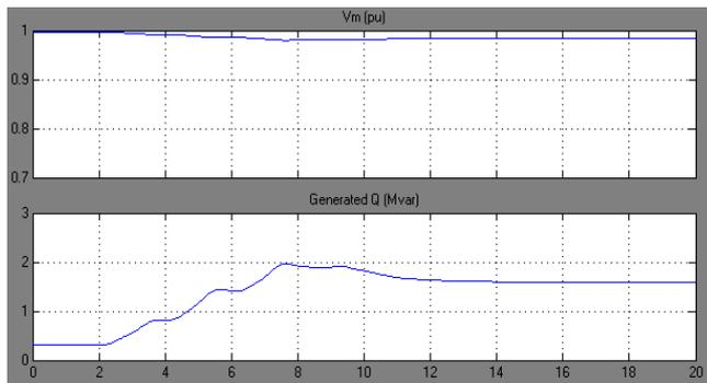
**Fig.16.**The injected voltage and reactive power by STATCOM for improvement of wind turbines operation
