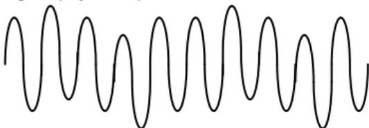
Fig.5.Voltage flicker of the system due to load variation
