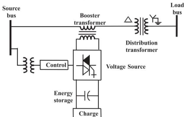
Fig.6.Basic structure of DVR
