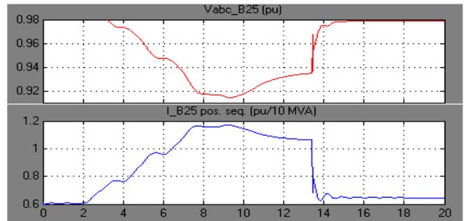
Fig.13. The voltage drop and current variation of analyzed bus 25 of system under wind turbine operation without STATCOM
