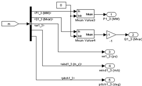
Fig.11. The subsystem of simulated system for data acquisition of wind turbines
