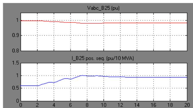
**Fig.17.**The improvement voltage and current of analyzed bus 25 under wind turbine operation with STATCOM
