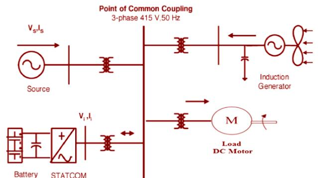
Fig.8.Basic structure of STATCOM at grid connected wind turbines
