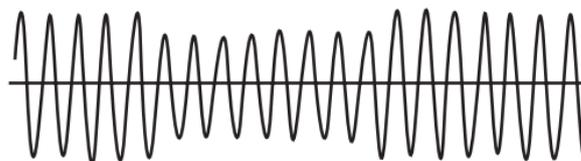
Fig.1.Voltage sag of the system
