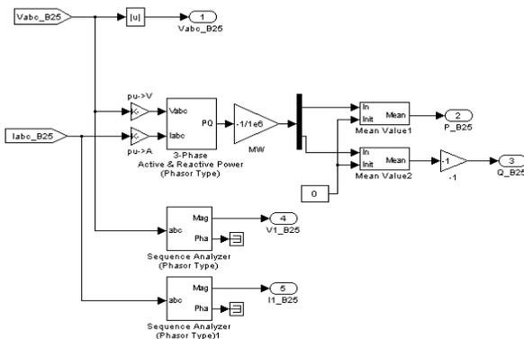
Fig.10. The subsystem of simulated system for data acquisition of analyzed bus
