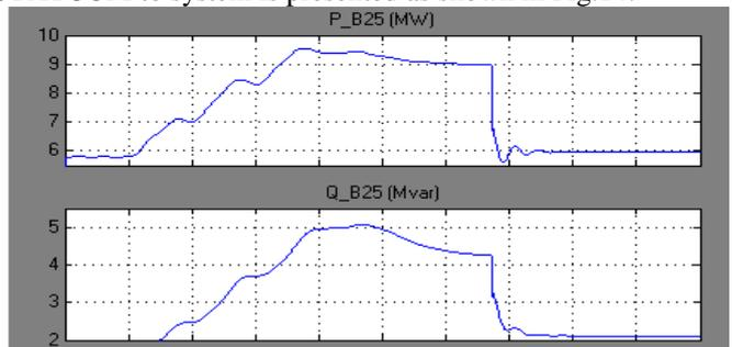
Fig.14. The variation of active and reactive power at bus 25 of test system
