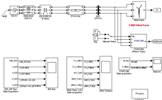
Fig.9. MATLAB/SIMULINK diagram of grid connected wind farm
