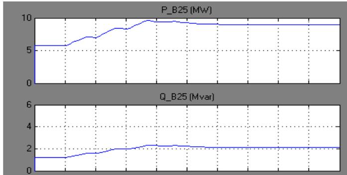
**Fig.15.**The variation of active and reactive power at Bus 25 of test system with presence of STATCOM
