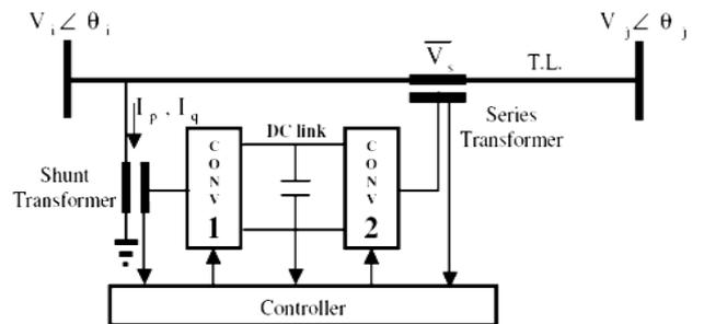
Fig.7.Basic structure of UPFC
