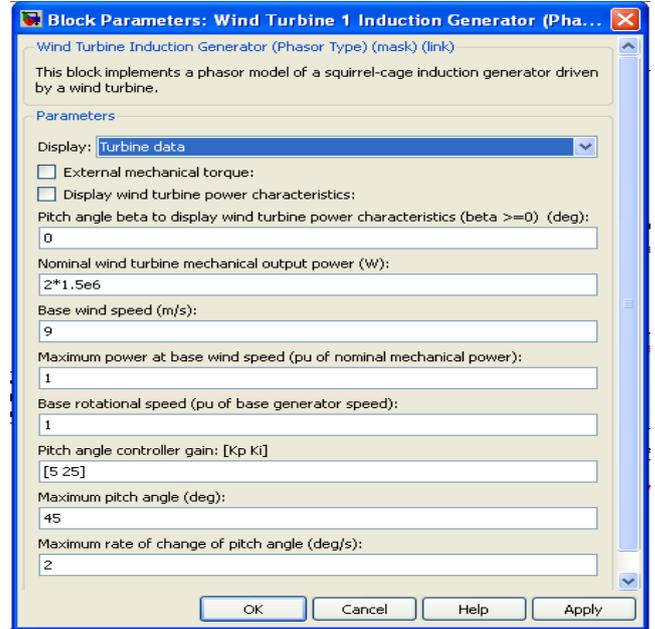
Fig.12. Setting of wind turbine parameters
